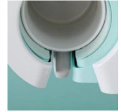
2. Ensure heat plate covers design.
